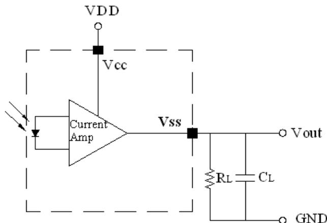
Figure 2 PDIC block diagram and recommend circuit
