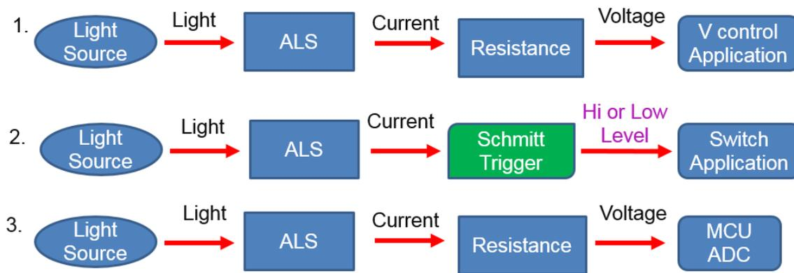
Figure 4 Light convert to electric application process
