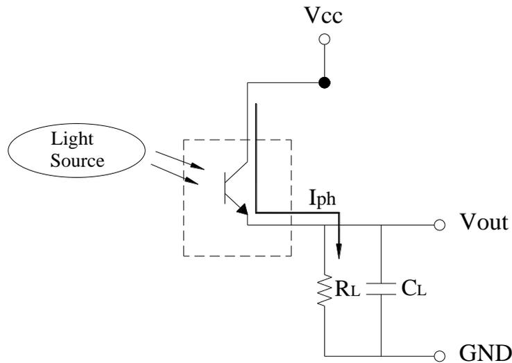
Figure 1 photo current convert into output voltage circuit
