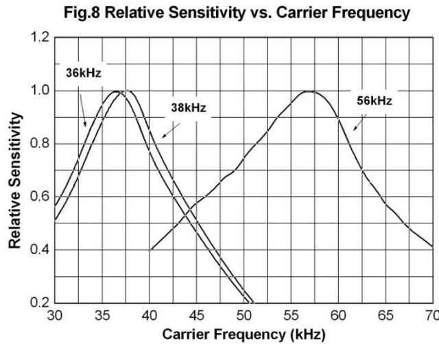
Figure 3. Support Carrier Frequency vs. Relative Sensitivity
