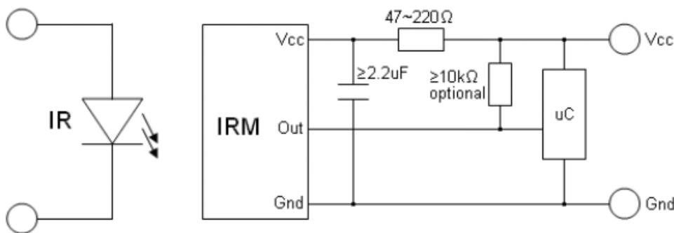
Fig 10. Reference circuit
