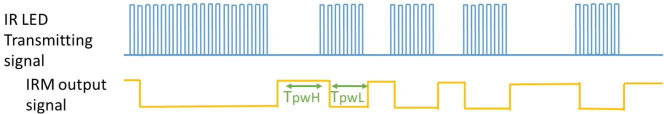
Figure 4. Infrared emission and Reception signals
