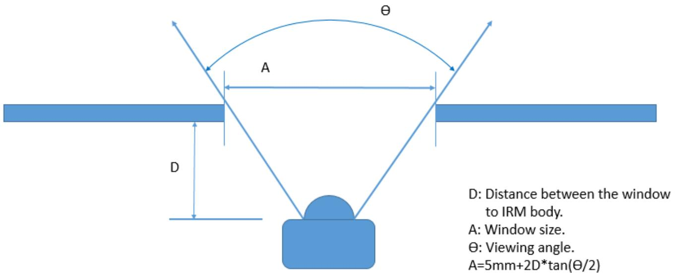
Fig 9. Mechanism illustration
