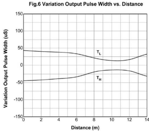
Figure 5. Variation Output Pulse Width vs. Distance
