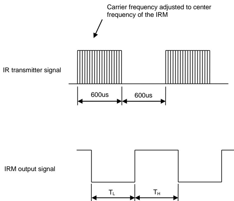
Figure 6. IR transmitter signal and IRM output signal
